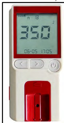
Figure A+1.2 Prestige stick test hemometer
