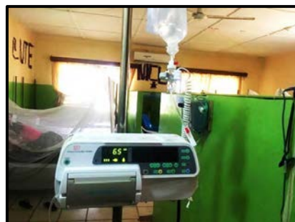
Figure B2. 2 Drip monitor infusion device for Safe intravenous administration of drugs Available from Diamedica
