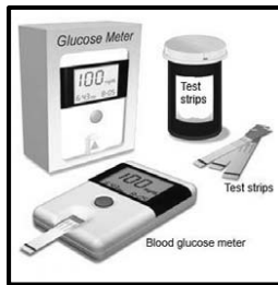
FIGURE 99.2 Electronic reading device for glucose strip. The strip is inserted into the side of the machine after the sample has been timed for the reaction to take place and the blood has been wiped off the strip.
