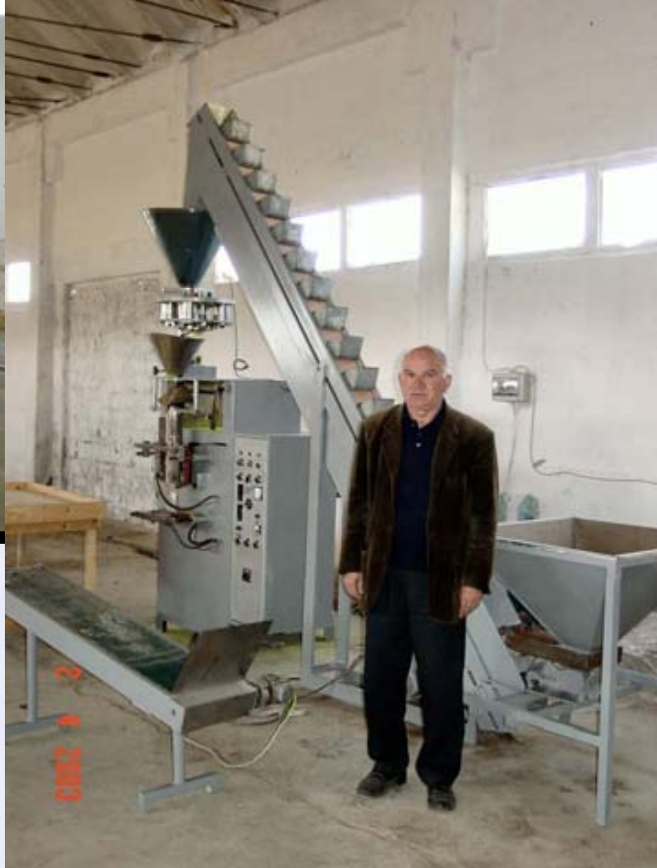
This is the equipment with which the salt is iodised and packed.
